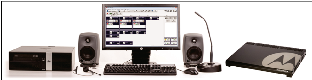
Figure 1 - 1: MCC 7500 Dispatch Console, including desktop PC, headset, speakers, display, keyboard, mouse, microphone, and voice processor module
