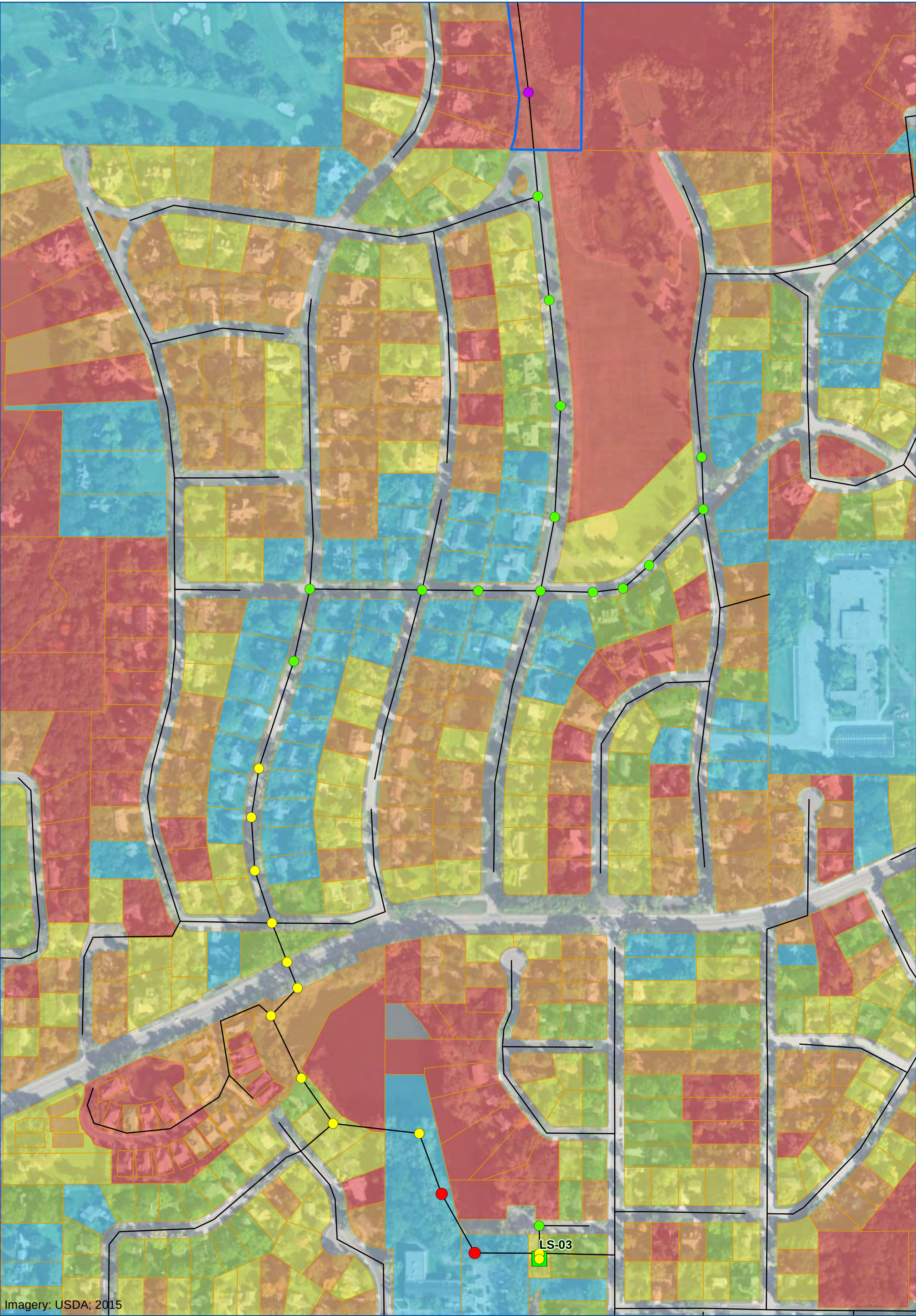
Timing and Location of Surcharged Manholes Related to Failure of Lift Station 3 City of Edina, MN FIGURE 19
