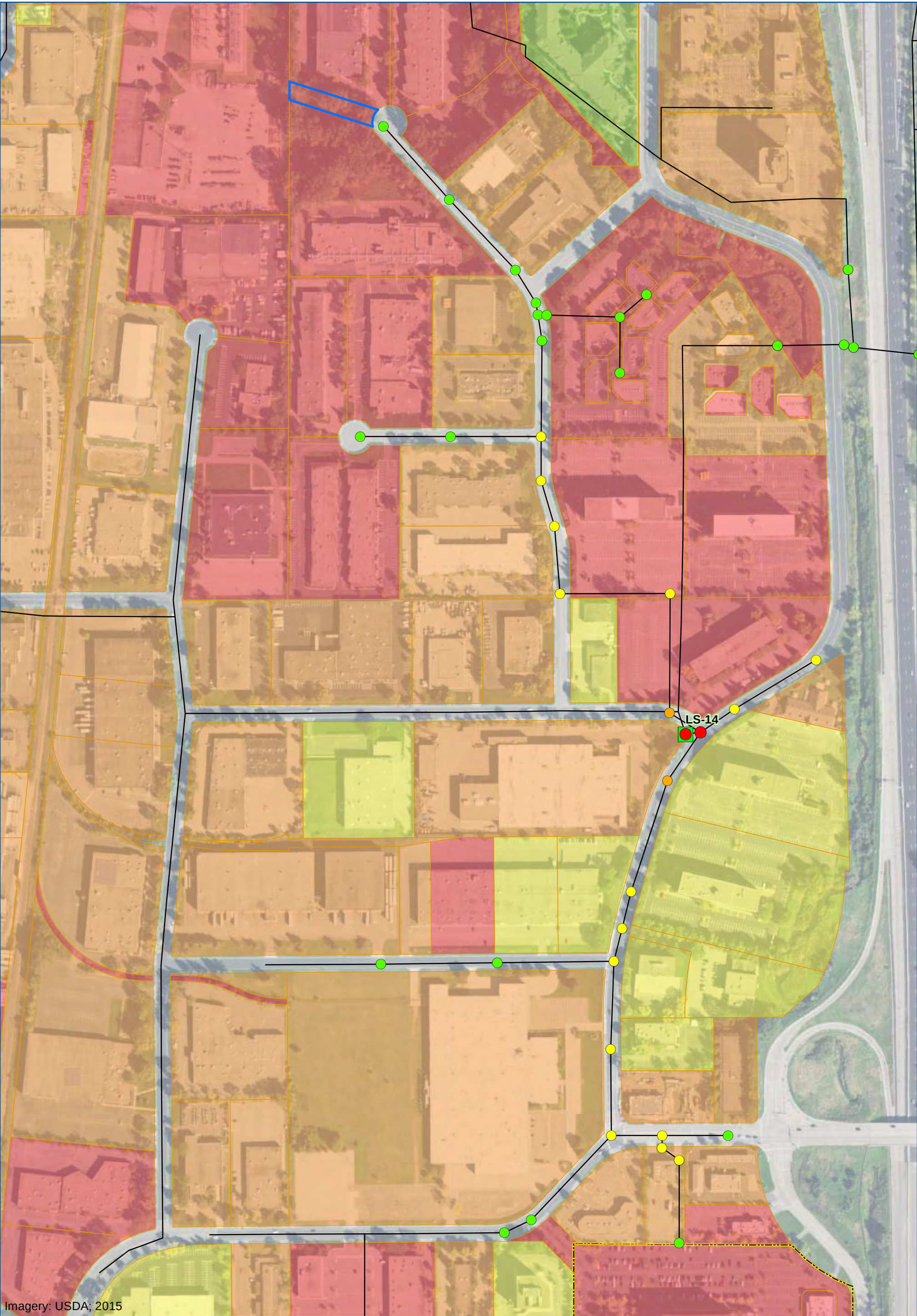
Timing and Location of Surcharged Manholes Related to Failure of Lift Station 14 City of Edina, MN FIGURE 14
